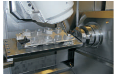
Figure 2: In tandem, CAMWorks and the Mazak Integrex machine the cylinder heads for peak engine performance
