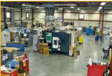
GEO-1119A: Tomak's 20,000 sq.ft. of manufacturing floor space includes four Swiss Machines and sixteen lathes
